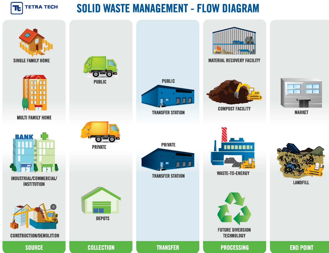
Figure 2-1: Solid Waste Management Flow Diagram
